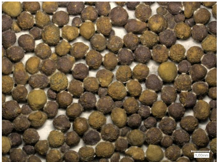
Novel particles bonded to a ceramic matrix composite substrate to be used in the high temperature abrasion test bench, which is currently under development
