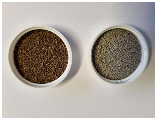
Figure 10. BL 16/30 particles before and after electroless nickel coating.
