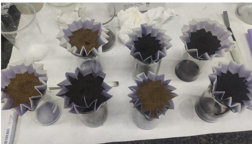
Figure 3. Particles located in a funnel with filter paper during coating process.
