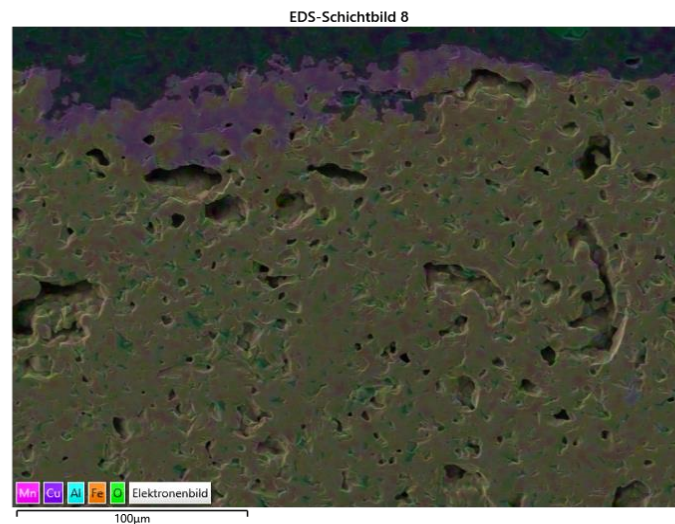
Figure 16. SEM/EDX mapping of deep black coated granulated gen3
