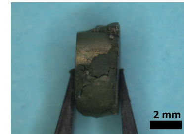
Fracture pattern for \text{Cr}_{92}\text{Si}_8 after compression test @ 700°C
