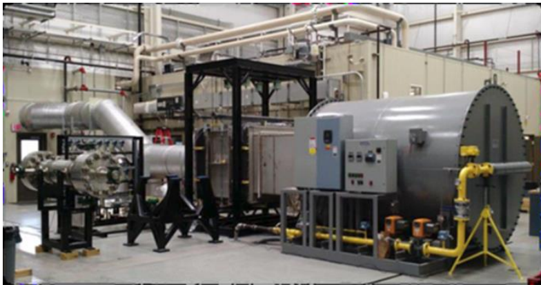
First fired sCO 2 system using 740H Sun Shot Turbine Test Heater (Thar/SwRI)
