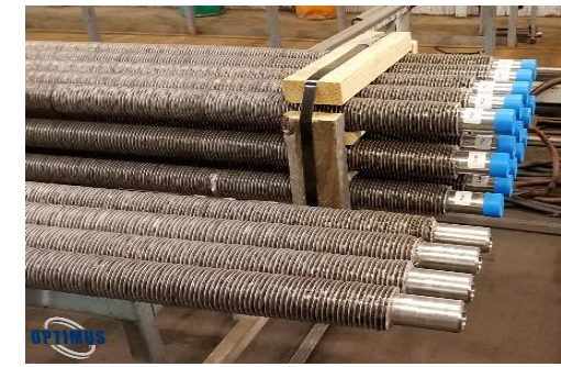
IN740H tubing with 304S fins
