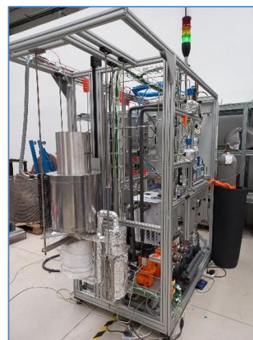
Figure 19. Supercritical Carbon dioxide Autoclave model with the description of the main components (left), the current state of the assembled device during the test operation (right).
