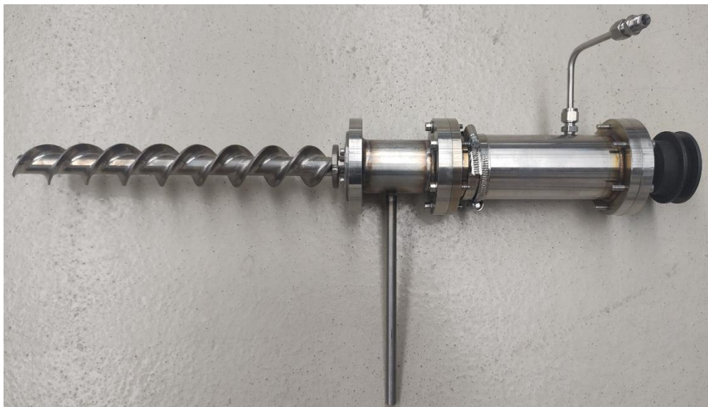
Figure 11: Fabricated screw conveyor assembly.
