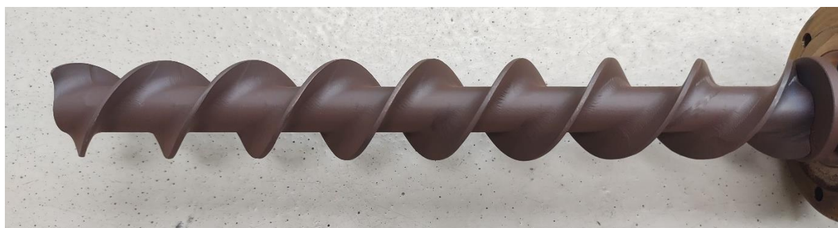
Figure 28: Screw conveyor after 40h of operation.
