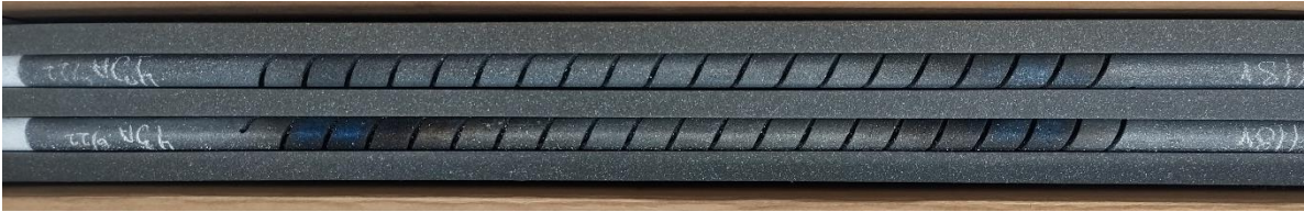
Figure 23: SiC heating elements from the last heating stage.
