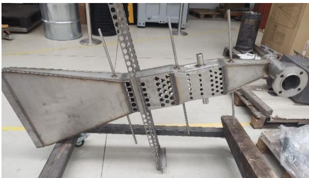
Figure 5: Newly fabricated test section for long term abrasion tests.
