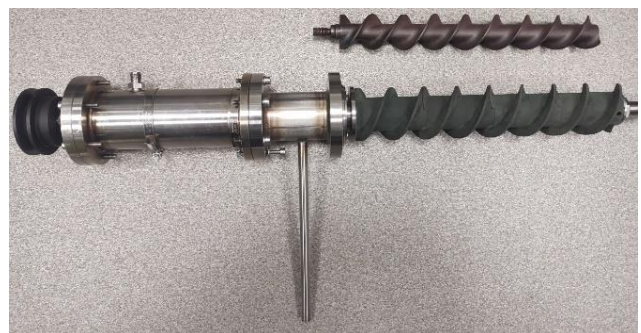
Figure 6: Comparison of new screw conveyor (3D printed from Inconel718 and heat treated) vs. old design.
