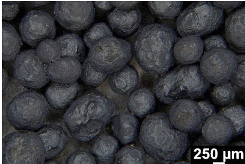
Figure 3. Initial state of Gen 4 particles with the DECHEMA coating (left). Gen 4 particles with the DECHEMA coating after more than 10 years simulated or more than 7300 impacts (right)
