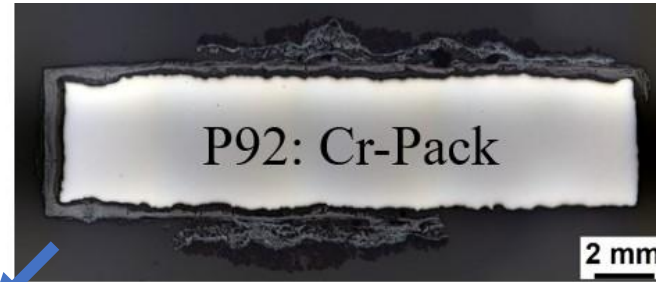
Samples covered with 10g of combustion ashes
