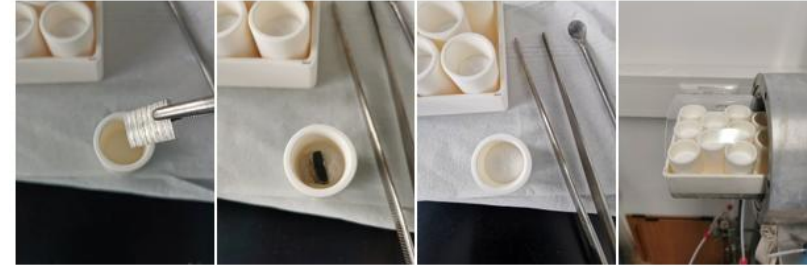
Samples covered with 10g of combustion ashes
