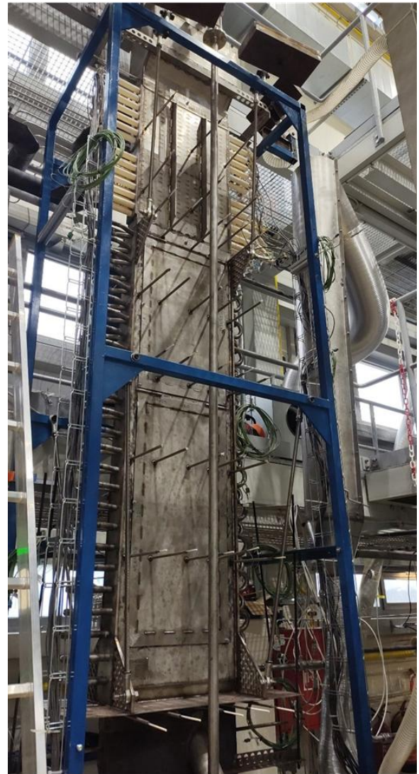
WP5 Final test rig – integrated particle/sCO 2 heat exchanger mock-up
