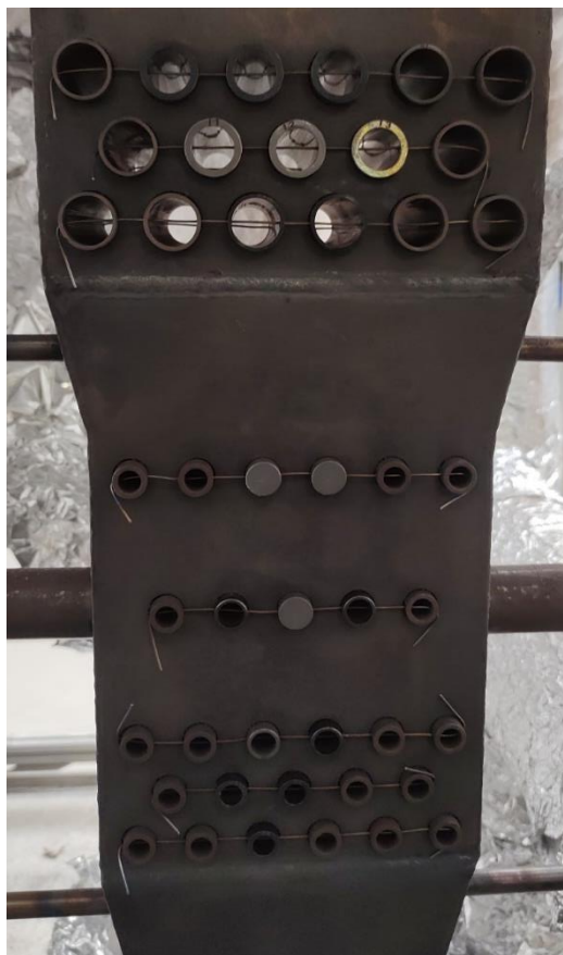
Figure 37: Test section with the tested material samples.
