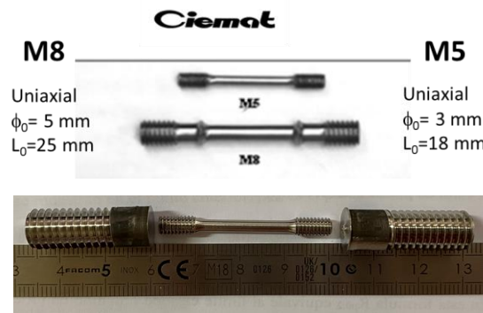
Figure 47. M8 vs. M5 specimen. M5 specimen machined from M8 specimen.
