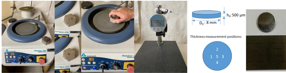
Figure 64. Finished procedure to obtain discs for SPC tests.
