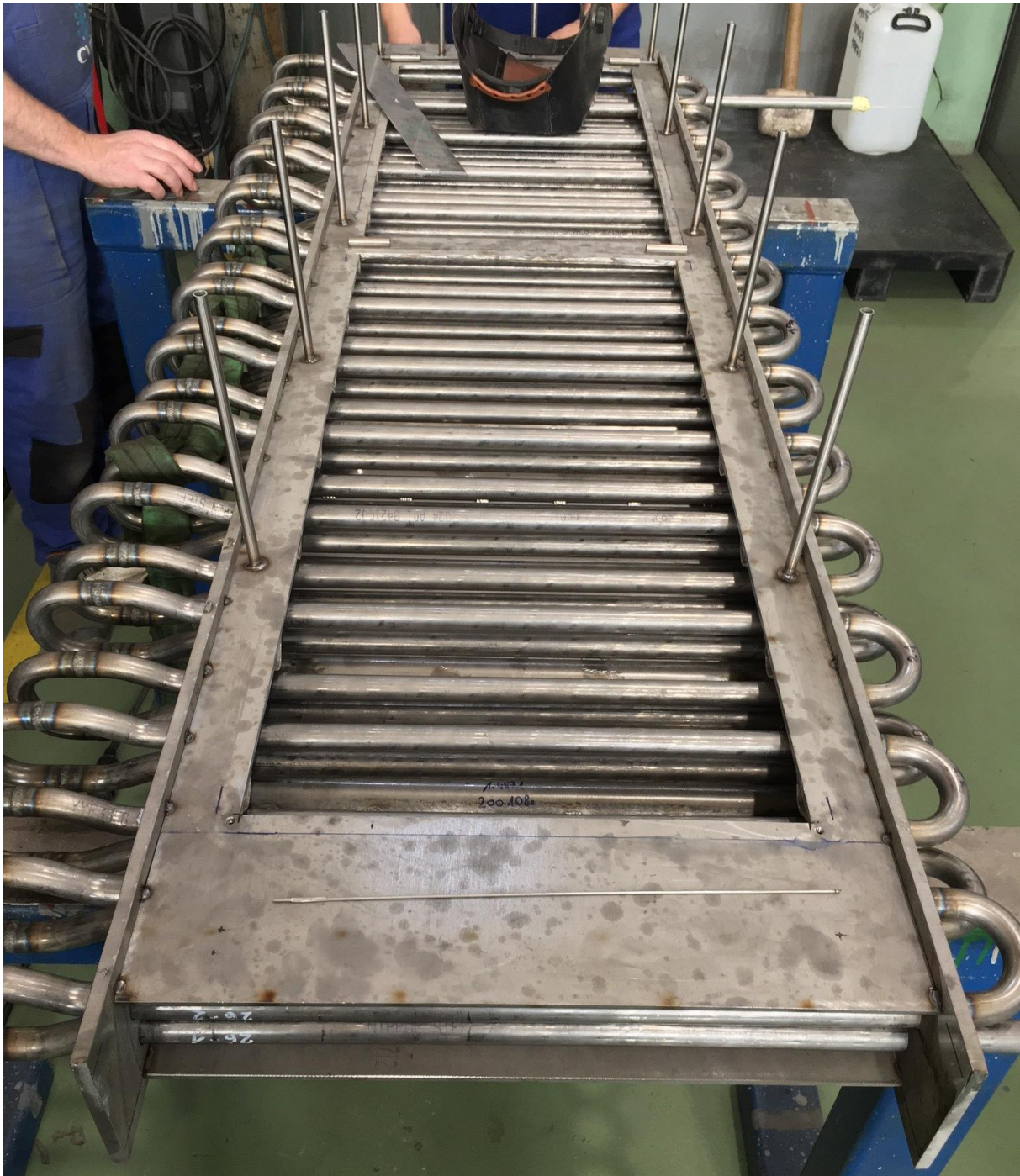
Figure 9: Heat exchanger during the fabrication - near completion.
